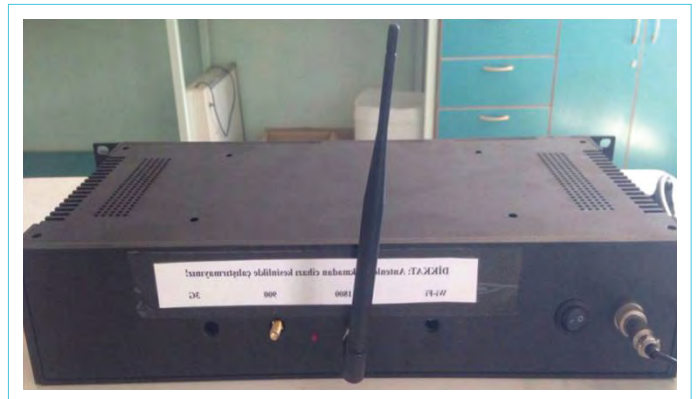
Figure 2. Transmitter (rf generator) operating at 900 MHz
