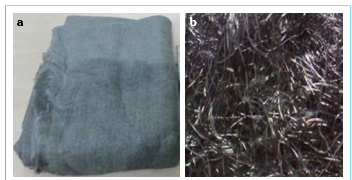
Figure 3. a, b. (a) EM field shielding fabric. (b) Microscopic view
